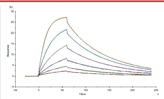
Human IL-2 R beta, Fc Tag (Cat. No. ILB-H5253) captured on CM5 chip via anti-human IgG Fc antibody, can bind Human IL-15, premium grade (Cat. No. IL5-H4117) with an affinity constant of 9.5 nM as determined in a SPR assay (Biacore T200) (Routinely tested).
