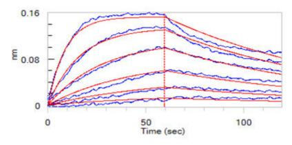
Loaded Human IL-2 R beta, Fc Tag (Cat. No. ILB-H5253) on Protein A Biosensor, can bind Human IL-15, premium grade (Cat. No. IL5-H4117) with an affinity constant of 10.2 nM as determined in BLI assay (ForteBio Octet Red96e) (Routinely tested).
