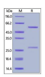
Biotinylated Anti-Cetuximab Antibody (AY31) on SDS-PAGE under reducing (R) condition. The gel was stained with Coomassie Blue. The purity of the
