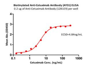
Immobilized Anti-Cetuximab Antibody (12B1E9) (Cat. No.CEB-Y29c) at 2  $\mu$ g/mL, add increasing concentrations of Cetuximab and then add Biotinylated Anti-Cetuximab Antibody (AY31) (Cat. No.CEB-BY31) at 1  $\mu$ g/mL. Detection was performed using HRP-conjugated streptavidin with sensitivity of 4.84 ng/mL (QC tested).
